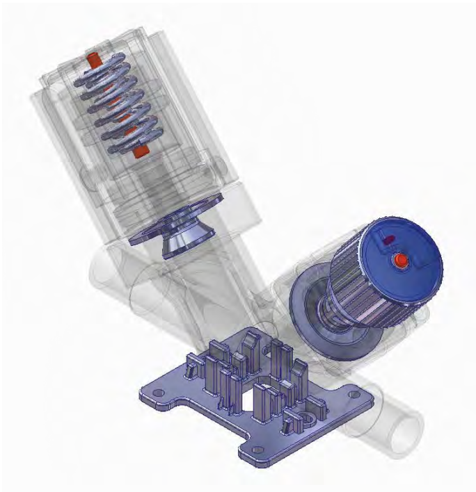
PMI Valve 조합 예 - 1 Pneumatic Valve + Manual Valve
