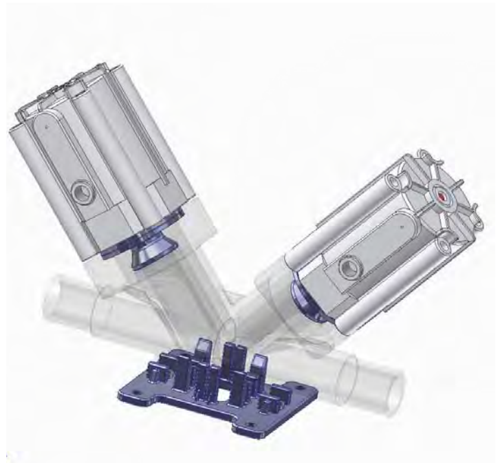
PMI Valve 조합 예 - 2 Pneumatic Valve + Pneumatic Valve
